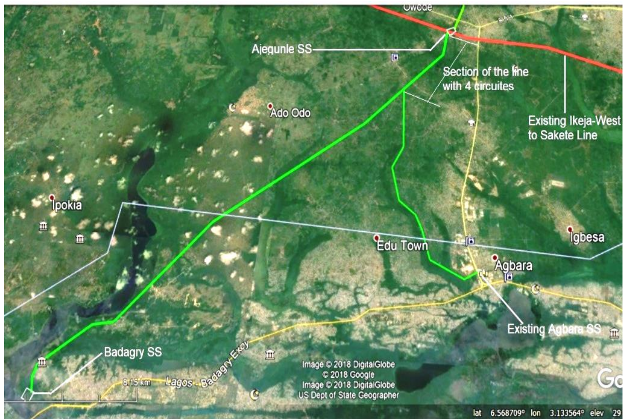
Figure 2.5 The 132kV Lines Showing Multi-Circuit Sections
